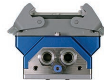
2.4 kW VCSEL module PPM412-12-980-24-c. 52 mm x 40 mm emission area in 12 separately programmable emission zones.
