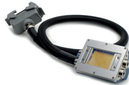
2.4 kW VCSEL module PPM412-12-980-24-c. 52 mm x 40 mm emission area in 12 separately programmable emission zones.
